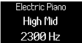
Controlling the High Mid-EQ band's frequency with encoder 5.
