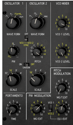
The two VCOs and pitch modulation controls
