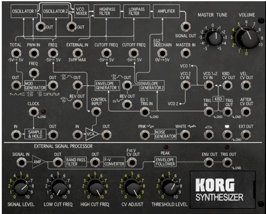
A complete KORG MS-20 synthesis voice, with the signal path and all modulators
