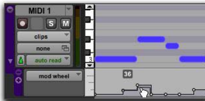
Stepped control automation
