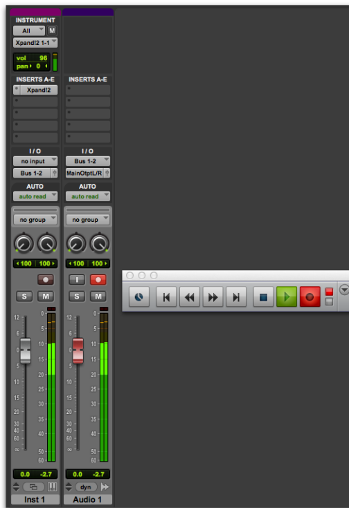
Bus recording audio from an instrument plug-in
