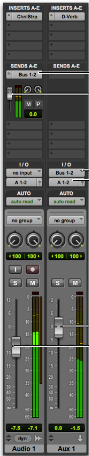
Send/return setup for an external device
