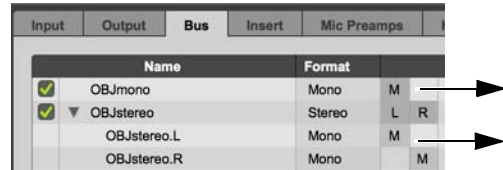
New mono bus and new stereo bus with mono sub-paths revealed
