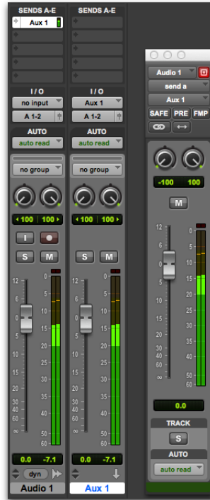
New Auxiliary Input track with audio track send automatically assigned to Bus 1–2
