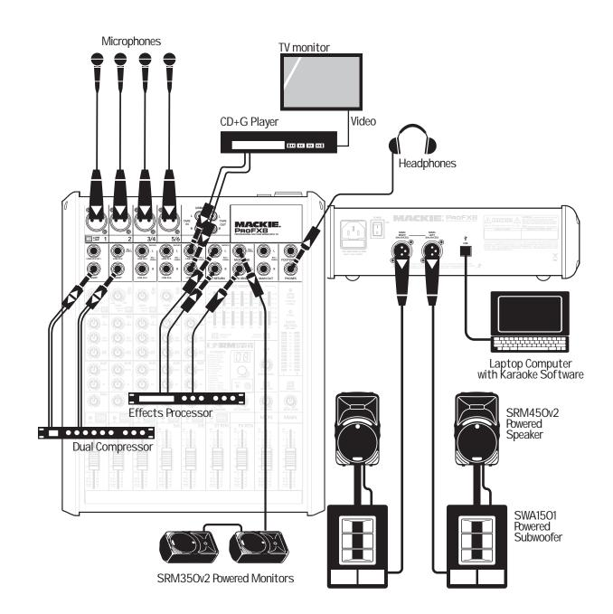
This diagram shows microphones attached to channels 1 to 4, and a CD+G player connected to the line-level inputs of channel 7/8. An effects processor receives a mono input from the FX send, and its stereo outputs connect to the stereo return inputs. A dual compressor is connected to the insert of channel 1, and 2, allowing vocal compression.
