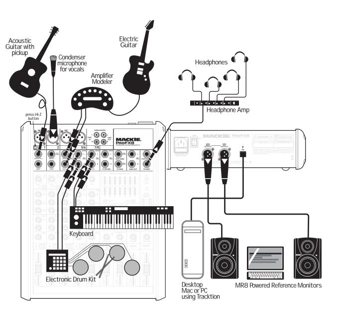
This diagram shows an acoustic guitar connected directly to channel 1 (with hi-z switch pressed in), a condenser microphone attached to channel 2 mic input, a guitar amplifier modeler connected to the line-level inputs of channel 3/4, an electronic drum kit connected to channel 5/6, and a keyboard attached to channel 7/8.
