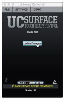
**WARNING:** Do not power off or disconnect your Studio 192-series interface during the firmware update. Once the firmware update is successfully completed, you will be alerted and instructed to reboot your device. Please make sure to close all applications before running the firmware updater.
