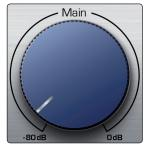
**Main.** The main knob controls the output level for the main outputs on the back of the Studio 192-series interface and has a range of -80 dB to 0 dB. This control provides attenuation only.
