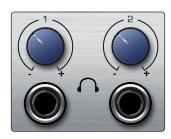
**Headphones Outputs.** Your Studio 192-series interface provides two/one headphone outputs, each with its own level control. Each headphone output is provided with its own unique output stream to route audio directly from your DAW (Studio 192: playback streams 11-12 and 13-14, Studio 192 Mobile: playback streams 7-8). From UC Surface, any mix can be routed to either headphone output.
