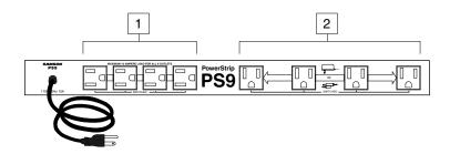
1: Switched AC outlets (horizontal mount) - Connect external equipment to these standard 3-pin AC outlets, which are turned on and off from the front panel Outlets switch (see #2 on the previous page).
