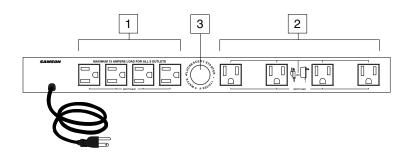
**1:** Switched AC outlets (horizontal mount) - Connect external equipment to these standard 3-pin AC outlets, which are turned on and off from the front panel Outlets switch (see #2 on the previous page).
