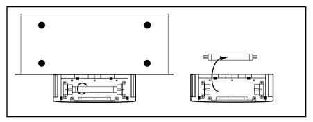
Follow the same procedure to insert a new bulb, then replace the clear plastic diamond lens by pulling gently back on both retaining tabs.
