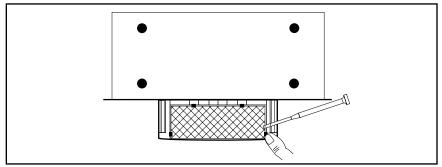
The bulb is now easily removed by giving it a half-turn so that its end terminals line up with the holder slots.
