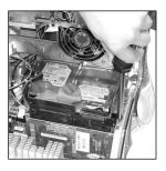
4. Insert the card carefully, and make sure that it is fitted properly into the slot.
