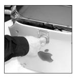
**3.** Remove the screw and the blind panel on the PCI slot you are planning to use.
