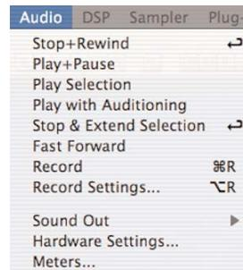
The Audio menu contains commands for playing back and recording audio, as well as configuring Peak's Recording Settings, your audio hardware, and Peak's Meters.
