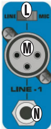
**M. MIC INPUT JACK** – Plug your microphone in here. This three pin XLR balanced female input connector is intended for input signals from low impedance microphones.
