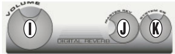
**I. MASTER VOLUME LEVEL CONTROL** – The master volume control adjusts the output volume of the P80. The master control features a notched position indicator. For the majority of applications the Passport system has been balanced to operate with this control at its notched 12 o'clock position. In situations where more volume is required the master control can provide an additional 6 dB of gain when turned to the right of the center position.
