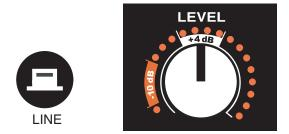
When a microphone, instrument or other consumer product is connected to the system, first ensure that the "LEVEL" control is at its minimum, anti-clockwise, OFF position. Then select the "Mic" input sensitivity and slowly increase the level. If the "overload" LED illuminates you should back the level down again. If the "overload" LED illuminates and the "LEVEL" control is barely cracked open then you should try selecting the "LINE" input sensitivity range.
