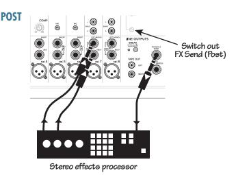
Using the output to feed a stereo effects processor. In this example, the stereo outputs go to ch. 7 stereo inputs.
