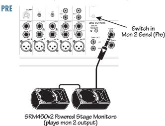
Using the output to feed a pair of powered stage monitors.
