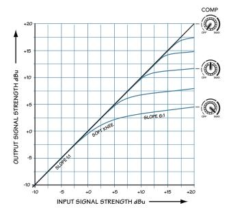
The other blue curves represent in-between positions of the compressor knob, with higher thresholds before compression begins.
