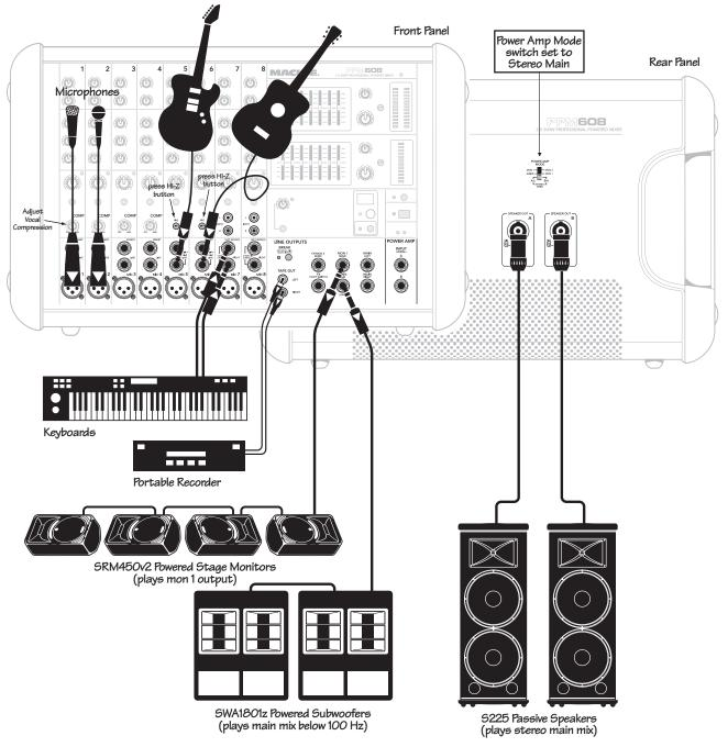
This diagram shows microphones attached to channels 1 and 2, electric guitars connected directly to channels 5 and 6 (with hi-z switch pressed in), and a keyboard attached to channel 7's stereo inputs. A portable recorder is attached to the stereo tape outputs to record the performance.
