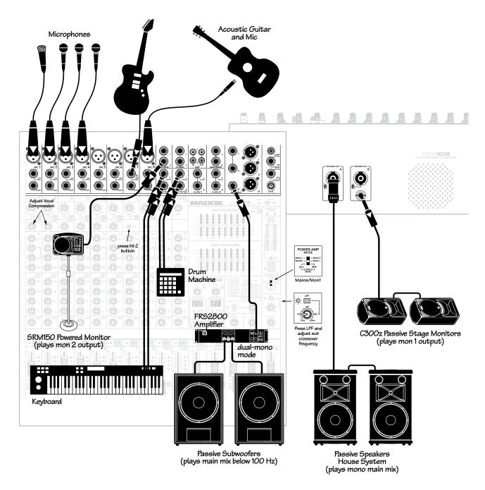
This diagram shows microphones attached to the mic inputs of channels 1 to 4, an electric guitar connected directly to channel 7 (with hi-z switch pressed in), an acoustic guitar microphone connected to channel 8 mic in, a keyboard attached to channels 9/10, and a drum machine to channels 11/12.
