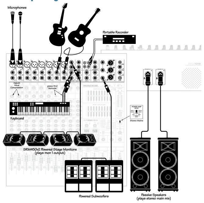
This diagram shows microphones attached to channels 1 and 2, electric guitars connected directly to channels 7 and 8 (with hi-z switch pressed in), and a keyboard attached to channels 9/10. A portable recorder is attached to the stereo tape outputs to record the performance.
