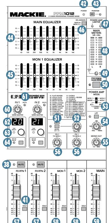
With this constant-Q graphic EQ, the bandwidth (and Q) of a frequency band doesn't vary with the amount of boost or cut, and the adjustment of one slider has minimal effect
