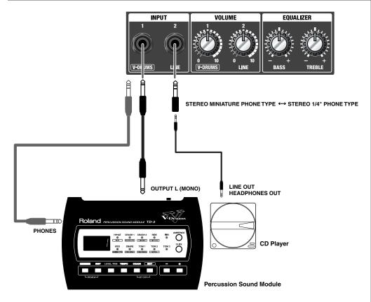
\* Once the connections have been completed, turn on power to your various devices in the order specified. By turning on devices in the wrong order, you risk causing malfunction and/or damage to speakers and other devices.
