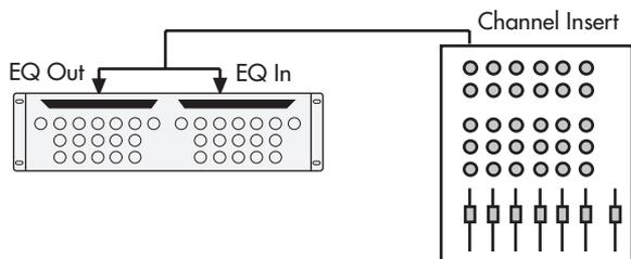
This example shows you how to connect the PEQ-450 to one mono source. You can use this method to connect two mono or stereo sources to the PEQ-450. You would need up to four insert cables to make these connections.
