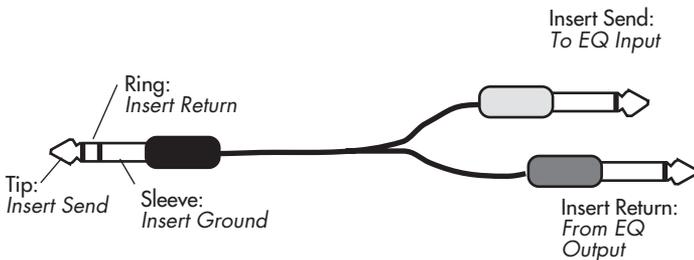
This cable splits the TRS insert jack into two unbalanced mono connectors. Usually, the tip is connected to the **INPUT** of the equalizer and the ring is connected to the **OUTPUT** of the equalizer. However, this may be reversed on some recording consoles. Check your mixer's Reference Manual to be sure or just try it both ways – this won't damage the PEQ-450.
