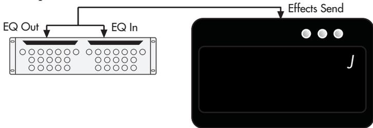
Another method would be to insert the PEQ-450 between the preamp and the power amp, if you are using a two-piece system. You should never put the equalizer between the power amp and the speaker, the high-powered levels created by the power amp will damage the unit.
