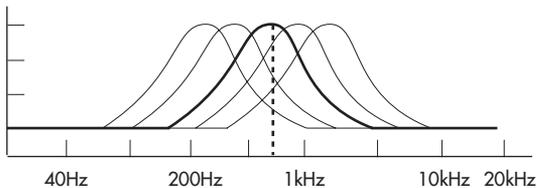
The Diagram above shows the effect of sweeping the frequency control up and down.
