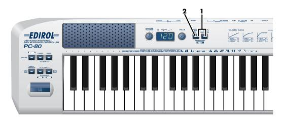
Simultaneously press the MIDI CH button and PGM CHANGE button.
