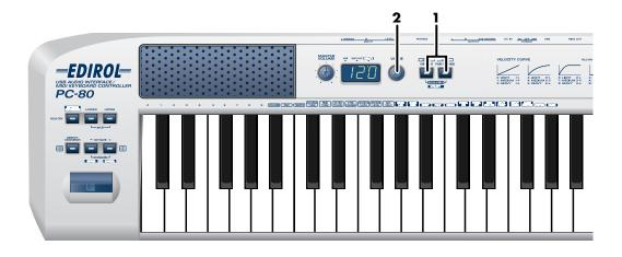
Simultaneously press the **MIDI CH** button and **PGM CHANGE** button.
