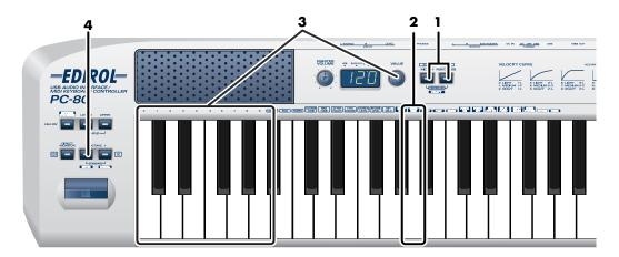
Simultaneously hold the [MIDI CH] button and [PGM CHANGE] button down.
