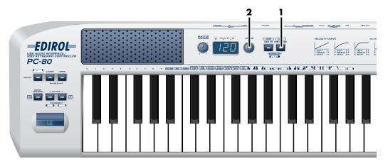
Make sure that the PC-80's **SOFTWARE SYNTHESIZER** button is not lit. If you're in Controller mode (p. 67), switch to Play mode.
