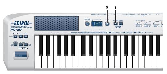
Make sure that the PC-80's **SOFTWARE SYNTHESIZER** button is not lit. If you're in Controller mode (p. 67), switch to Play mode.
