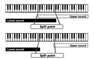
The Lower sound extends from the leftmost key to the specified key. The Upper sound extends from the rightmost key to the specified key. These keys are the **split points**.
