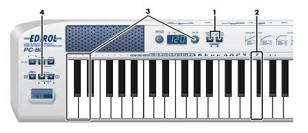
Simultaneously press the PC-80's MIDI CH button and PGM CHANGE button, and hold them down. The PC-80's display will indicate "UTL".
