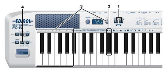
Simultaneously hold down the **MIDI CH** button and **PGM CHANGE** button for a few moments.
