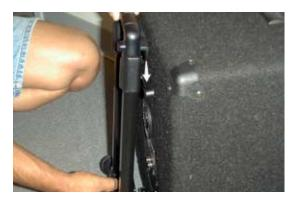
Next, press down on the spring-loaded tab on the bottom lip of the handle. While holding the tab down, line up the bottom lip underneath the lower bracket. When the handle is flush with the back of the cabinet, release the spring-loaded tab. The bottom lip will slide into the lower bracket.
