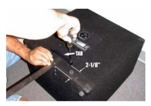
Install the remaining bracket (B) using the three remaining 6-19 x 1" screws (D) in the location shown. The "tab" should point towards the bottom of the cabinet. The top edge of the bracket is to be 13" from the bottom edge of the other bracket. Center the bracket horizontally by using the center screws on the jackplate as a reference.
