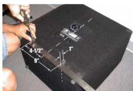
Install one of the brackets (B) using three of the 6-19 x 1" screws (D) in the location shown. The "tab" should point towards the top of the cabinet. The bottom edge of the bracket is to be 2-1/8" from the bottom of the cabinet. Center the bracket horizontally by using the center screws on the jackplate as a reference.
