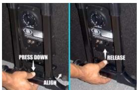
Press down on the spring-loaded tab on the top of the handle and raise the handle until it locks into its fully extended position. Pull back on the handle to tilt the cabinet onto the rollers, and GO!
