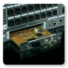
The X32's expansion slot provides flexible and expandable connectivity for many different applications. The X-MADI Expansion Card can easily be installed in place of the X-USB card that is included with the X32. The 32-channel interface brings even more I/O options to the X32 by instantly enabling it for MADI networking. The MADI or AES10 protocol is quickly becoming an industry standard in many broadcast applications.
