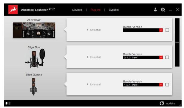
Open Antelope Launcher and click the 'Plug-ins' tab. Click the checkmark in 'AFX2DAW', then click the 'update' button to download and install the plug-in.
