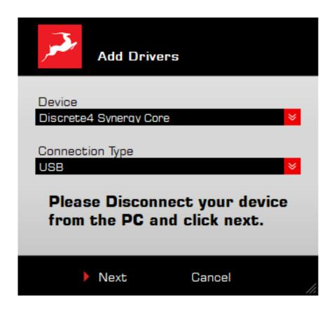
Choose your device and connection type from the drop-down menus, disconnect the device from your computer, and click 'Next' to perform a driver re-install.
