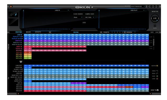
Welcome to the Orion 32+ | Gen. 3 Core software Control Panel! More than just an alternative to the physical front panel controls, it provides intuitive and comprehensive access to each aspect of the converter's functionality. This includes settings, signal routing, audio mixing, effects, presets and more.
