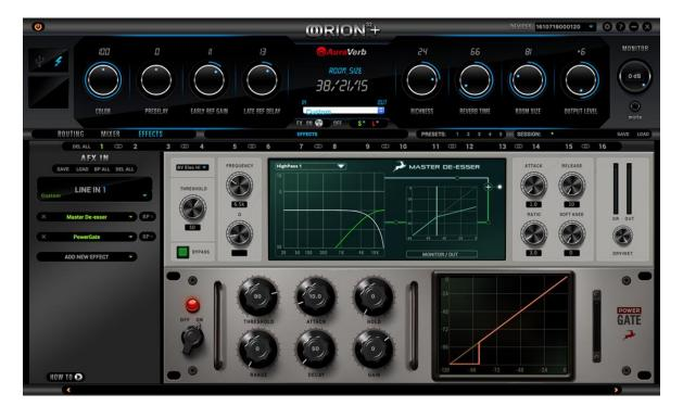
The 'Effects' tab lets you apply up to 8 FPGA FX per mono audio channel for a total of 16 channel strips and 128 FX instances, independent of sample rate. However, different types of FX place different processing loads, resulting in the following instance limitations:
