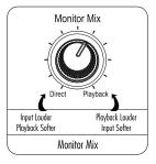
**NOTE:** This does not change the recorded volume, only what you hear while you are recording. You can also adjust the playback level and pan position of the original track in your monitor by adjusting the contols for Channel 1 on Cubase's Mixer window.
