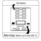
Now check the meter on the front of the Omega to make sure you are not clipping. If you want to hear the mic in headphones, turn up the Omega's Output Level control and turn the Monitor Mix control left (towards the Direct side).
