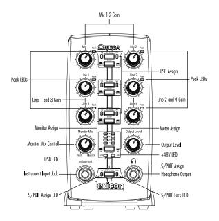
For the cleanest recording, adjust the Gain knob so the microphone level reaches at least "-6" on the meter, but never hits "Clip", on the loudest sound you'll be recording. If you see the PEAK LED on constantly. turn the Gain knob down until it flashes only occasionally, on the peaks.
