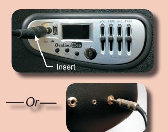
The analog circuits in the preamp are activated by either inserting stereo headphones into the headphone jack or by connecting your guitar to an amp or PA with a 1/4" instrument cable.
