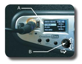
Scroll the screen cursor (A) by moving the joystick (B) up or down until it highlights the **TUNER** selection on the menu. Then navigate to the tuner by moving the joystick to the right or by pushing in.
