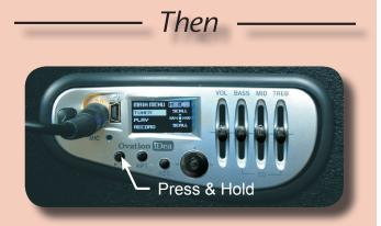
Turn on the preamp's digital functions and display window by pressing and holding the (Play/Stop) button for two seconds. Upon release, the player will boot and bring you to the MAIN MENU.
