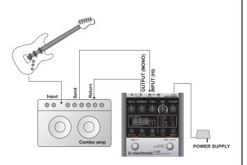
This example shows how to connect your NOVA Repeater pedal as a send/return effect in an effects loop. This is the correct approach if you use the pre-amp section of the amp to generate overdrive.
