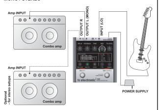
This setup illustrates how to use NOVA Repeater in a mono setup (one amp only) or in a stereo setup (two amps). Effects such as reverb and delay are usually placed as the last signal processors before the amplifier. Therefore, you should place all drive and modulation effects prior to NOVA Repeater.
