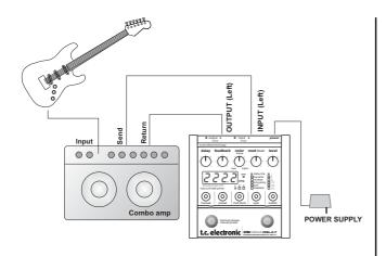
This example illustrates how to connect your Nova Delay pedal as a send/return effect in an effects loop. This is the correct placement of the Nova if you use the pre-amp section of the amp for overdrive sounds.
