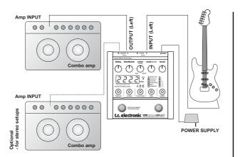
This setup illustrates how to use the Nova Delay pedal in a mono setup (one amp only) or stereo setup (two amps). Effects as reverb or delay are usually placed as the last effects before the amplifier. Therefore, - place all drive and modulation effects prior to the Nova Delay pedal.
