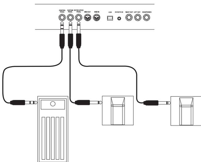
The Nord C2 Combo Organ has three pedal inputs; one for a sustain pedal, one for a rotary speed controller and one for a swell pedal.
