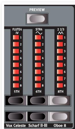
The buttons are special in the way that they auto-increment/ decrement the drawbar value when held. If you hold a drawbar button the corresponding drawbar value will continue to increment or decrement (within its range) until you release the button.
