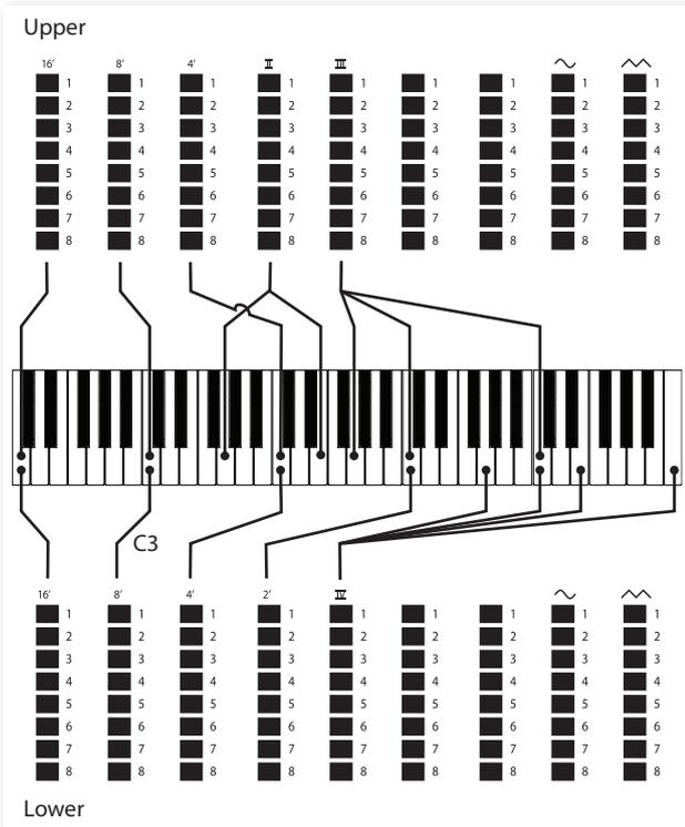
The two right most drawbars control the sum of all partials in the form of a filtered triangle-like signal sounding soft and dark, and an unfiltered square signal sounding bright and intense.
