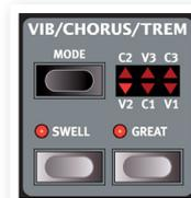
Three different types of choruses (C1- C3) and three different types of vibratos (V1-V3) are available. Select one of these types by pressing the Mode button. The effect can be activated/deactivated for both manuals individually by pressing the Vibrato/Chorus button for the swell and great drawbars
