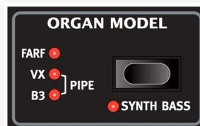
You select which model to play using the Organ Model button. Only one model can be used at a time.
