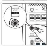
You can now control the preamp level and phantom power for your NSB stage box from the Fat Channel on your console, in the same way that you control the local inputs.
