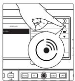
**Power User Tip:** In applications where you are using multiple NSB-series stage boxes of the same model, you can press the Identify button. This will flash Power / Network LED on the top panel red and green on the currently selected NSB, allowing you to quickly locate your selection.
