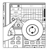
After you have set the preamp levels, enable Gain Compensation from the LCD. This will turn on Gain Compensation for that input and allow other mixers on the network to source that stream.
