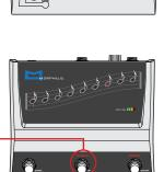
Press/release the TOGGLE switch to switch back and forth between the drop tune setting and the unaffected guitar signal.
