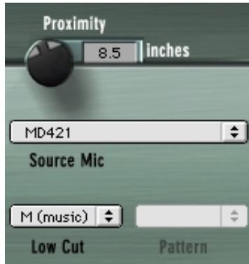
The SOURCE MIC section is where you specify the mic and the settings that were (or will be) used to capture the input sound. The purpose of these selections is to remove the effect of the source microphone, resulting in the signal that would have been recorded by an ideal instrumentation microphone with no proximity effect.
