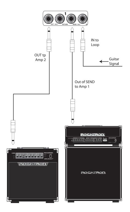
This connection diagram shows one way to use the PatchMate's buffered connection.
