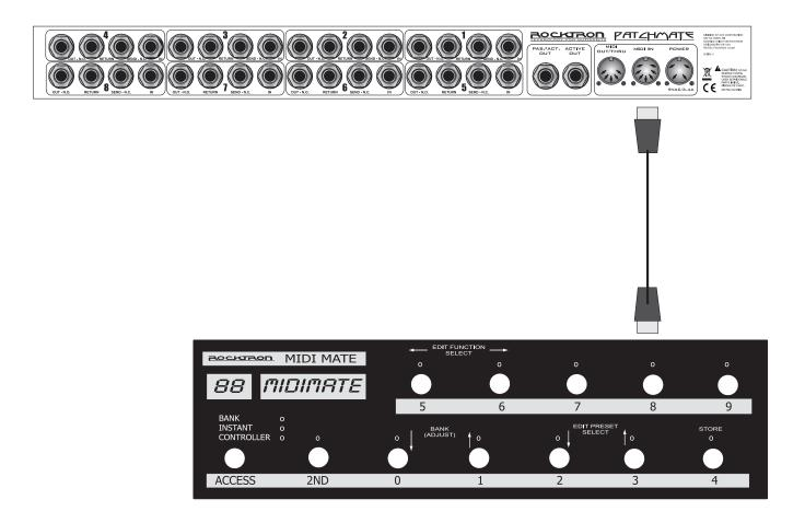
The PHANTOM POWER feature is provided exclusive to support all ROCKTRON MIDI CONTROL-LER products. Please refer to your owners manual before attempting to use this option with a MIDI CONTROLLER other than a Rocktron product. Rocktron can not be held responsible for any damages arising from improper use or connections.
