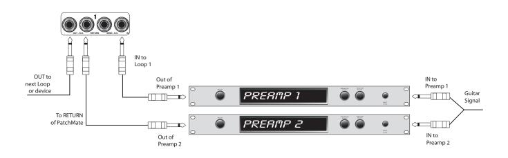
This connection diagram shows one way to use the LOOPs in the PatchMate to connect two amplifiers and select between the two.
