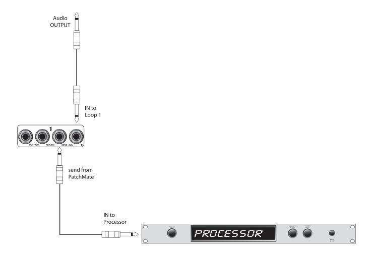
This connection diagram shows how to connect the PatchMate to a MIDI Controller such as the Rocktron MIDI Mate (use similar connections for the Rocktron All Access, All Access LTD and MIDI Xchange.
