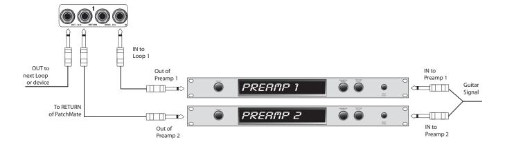
This connection diagram shows one way to use the LOOPs in the PatchMate to connect two amplifiers and select between the two.
