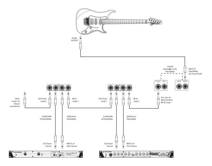
This connection diagram shows one way to use the LOOPs in the PatchMate to connect stompboxes (pedals). Although only two connections are shown here, you can follow a similar progression of connects using LOOPs 3-8.
