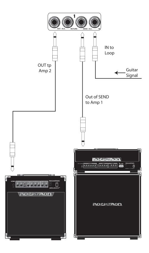
This connection diagram shows one way to use the PatchMate's buffered connection.
