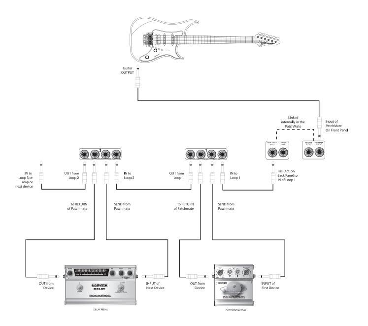
This connection diagram shows one way to use the LOOPs in the PatchMate to connect to multiple effects processors.
