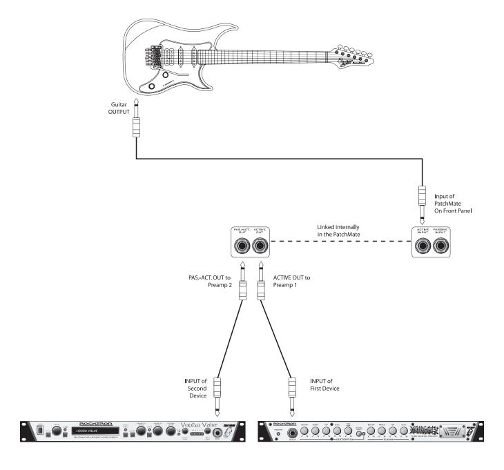
This connection diagram shows one way to connect the PatchMate to "MUTE" an effects processor where parallel effect routings are being implemented.
