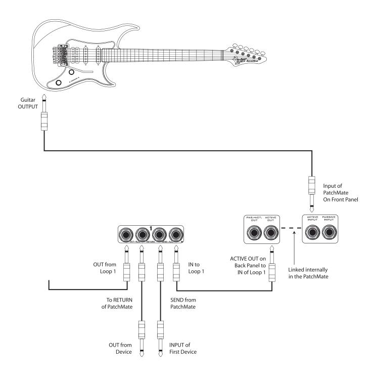
This connection diagram shows one way to use the PatchMates buffered connection to connect to two different preamps.
