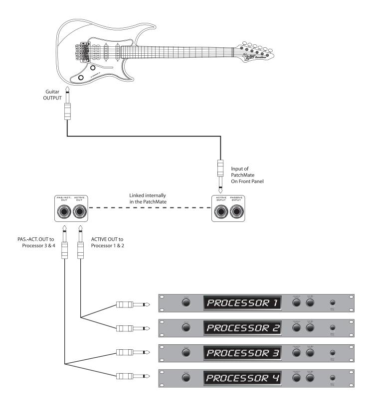
This connection diagram shows one way to use the LOOPs in the PatchMate to connect to two different preamp.
