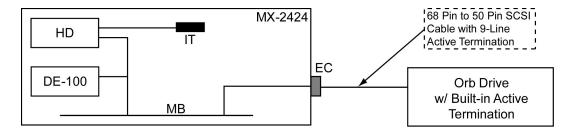
4. MX-2424 with stock internal hard drive, Rhino Jr. in the option bay, and external Orb Drive:
