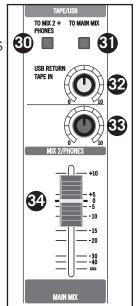
**34. MAIN MIX Fader -** The MAIN MIX Level fader adjusts the level of main left and right stereo mix sent to the MAIN MIX outputs.
