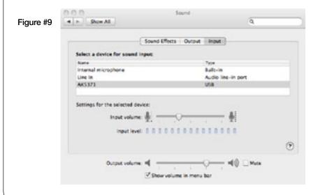
7. By watching the movements of the Input level meter in this window, you can now see that the Acoustica MVS USB microphone is working as you speak into it. This setting will be saved as the default input whenever the microphone is plugged in.
