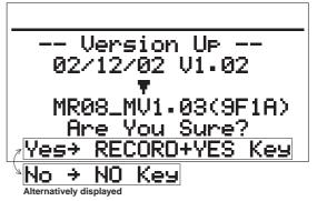
10) If the screen on your MR-8 matches one of the before listed examples, press the CURSOR RIGHT / YES / +1 ( $\circledcirc$ ) keys while holding down the RECORD key to start updating the software.
