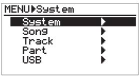
4) Highlight "USB" using the [CURSOR®] key and then press the [ENTER] key or [CURSOR®] key. MR-8 enters the USB mode, while the display shows the screen on the right.
