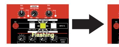
11) After updating the software is completed, the screen below with "Completed!" message will be displayed on the LCD. At the same time, both the insert effect MIC SIMULATION CONDENSER and TUBE keys are lit solid in green indicating that the program on the Flash ROM inside MR-8 is correctly erased and written.
