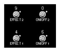
Press the button assigned to the desired relay state and hold the button down for two seconds. The relay state (for example, CH1) will flash once on the MPX R1 display to indicate that it has been stored with the program.
