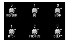
Buttons 1, 2, 3, 6, 7 and 8 bring MPX 1 effects (Pitch, Chorus, Delay, Reverb, EQ and Mod) in and out of bypass. The LED for each button indicates the current state of the MPX 1 Effect:
