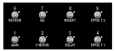
Buttons 1-4 and 6-9 bring MPX G2 effects (Gain, Chorus, Delay, Effect 1, Reverb, EQ, Insert and Effect 2) in and out of bypass. The LED for each button indicates the current state of the MPX G2 Effect:
