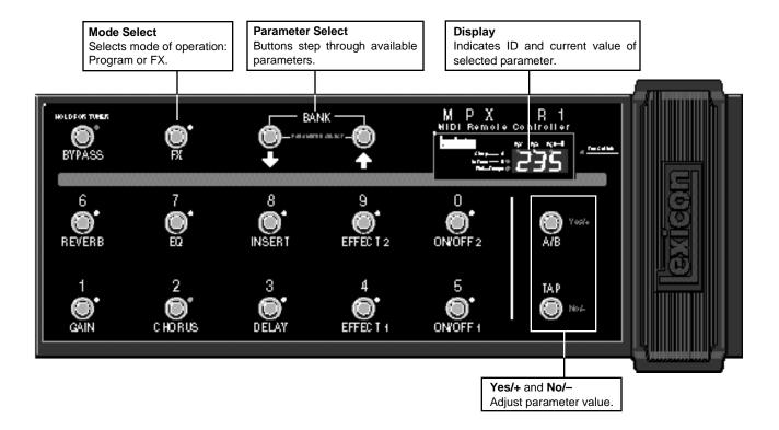
In either mode, the front panel BANK/Parameter Select buttons will step through the list of available parameters. The abbreviated name of each parameter will flash alternately on the display with the current parameter setting.
