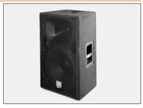
reinforcement of speech. The Laminar Flow Baffle reduces diffraction effects and distortion resulting from turbulence. The horn design with its large mouth delivers smooth, natural reproduction - especially in the critical midrange. The edges of the premium grade carpet are captured by the joint detail to prevent visible seams or peeling. A 16 gauge, steel grill protects the 15 inch JBL woofer.
