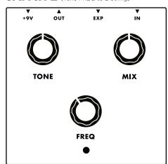
TONE - A filter circuit only applied to the effected signal. This allows you to leave in the MF Ring's natural high frequency chime and buzz, or dial it down for a warmer, more musical character. Because the tracking of the MF Ring is so accurate, this control is particularly useful for dialing in sounds that accompany lead lines, bends, and even chords. It is the perfect way to add unique texture to an idea without it overtaking the sound of your instrument.
