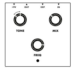
FREQ - Tunes the frequency of a carrier oscillator to the root note in a scale. The range of this control has been refined to be extremely musical. At lower settings chorus and octaves occur on notes within a chosen scale, while beating and extreme dissonance occur on notes played outside of that scale. At Mid position the sound is buzzy and tight. This is great when paired with drive for octave-fuzz sounds. At the maximum position the sound is much more synthesized and robotic.
