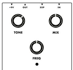
**EXPRESSION PEDAL INPUT -** This input is assigned to the Freq control. Use it to specify two independent playing keys or create classic sci-fi swells, bit reduction effects, and whammy dives. This input is additive and will allow you to go past the panel settings.
