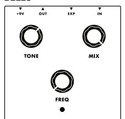
MIX - Sets the amount of input versus modulated signal. A ring modulator outputs the sum and difference frequencies of your instrument and the carrier oscillator (FREQ). At lower to medium levels, the MF Ring can be used to accompany and accentuate notes. As Mix is increased, you will notice more synthesized and bell-type sounds. At maximum, the input signal is completely gone and only sum and difference frequencies are heard. This is perfect for creating wild robotic and electric sounds.
