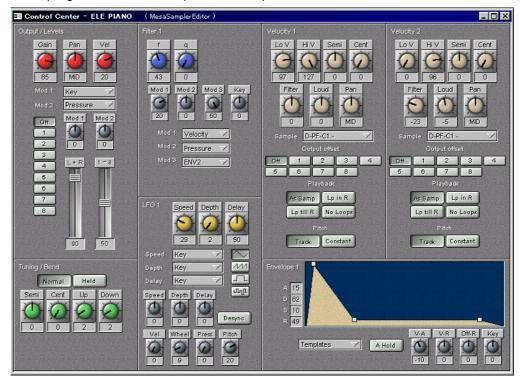
The Control Center Window is divided into the several sections, and the pop-up menu with a right-click at each section lets you choose the section to edit. For example, the top left section can be used as either "Output & Levels" or "MIDI Setup".
