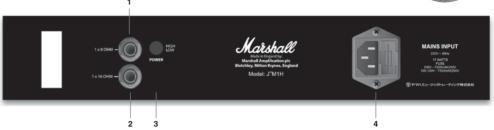
**WARNING:** Although your JTM-1 amplifier has two extension speaker outputs, never attempt to connect cabinets to both extension speaker outputs simultaneously. Only use one speaker output at a time.
