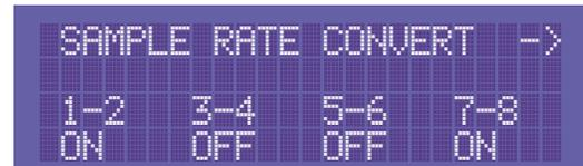
3. Press the **Select** button corresponding to the desired input channel(s) and toggle the selection. **On** enables sample rate conversion, **Off** disables it (default).
