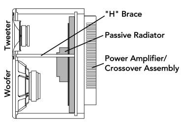
Figure 1. HR824 Cutaway side view
