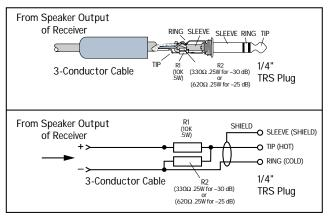
Figure 4. Speaker-level to Line-level TRS Pad
