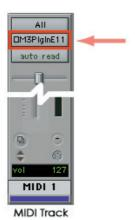
To route the M3's audio signal to Pro Tools LE 7, create an audio track or an AUX input track. As the input, select the audio interface input to which you've connected the M3's audio signal.
