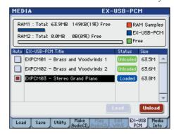
*Note:* If there is free space in both RAM1 and RAM2 (if the EXB-M256 is installed), the data will be loaded starting with RAM1.
