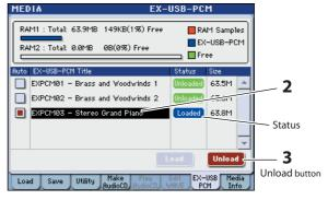
3. Press the Unload button. A dialog box will appear, so press the OK button to unload the data.
