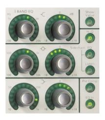
The Liquid Channel<sup>TM</sup> features a new digital ('modelled' rather than 'convolved') EQ, loosely based on the classic Focusrite sound of the original ISA 110. This is designed to allow small amounts of corrective shaping. All of the EQ settings can be saved, along with those of the mic-pre and compressor, in one of the Program slots (see the DATA SELECT section below).
