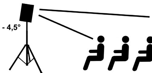
At events with a seated audience and rooms with smaller dimensions, it is advisable to select a downward angle. This way, in addition to a short-range acoustic cover, adverse reflections on low ceilings and rear walls are minimised.
