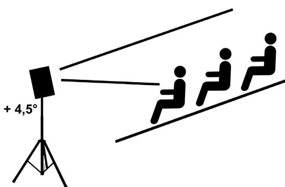
To obtain an optimal dispersion in a pedestal sound situation, choose an upward angle.
