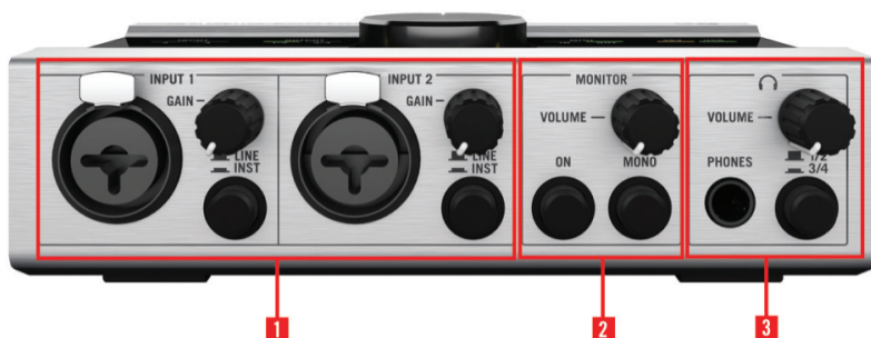
5.1 The front panel of the KOMLETE AUDIO 6.
