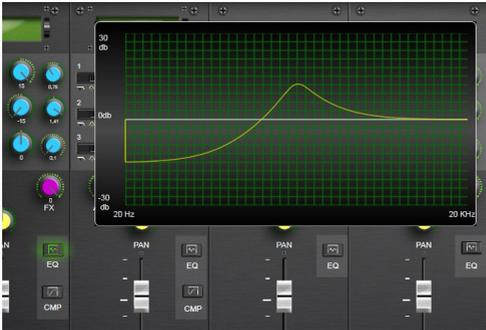
This windows shows a graph where the user can intuitively see the effect of the corresponding filter on the signal frequency spectrum.
