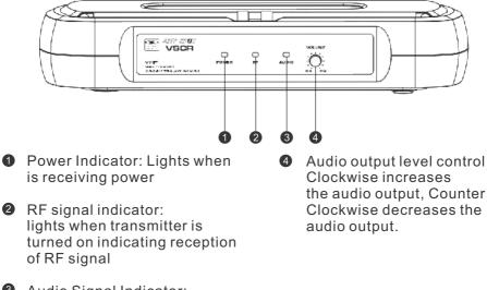
Audio Signal Indicator: Lights when receives audio from transmitter
