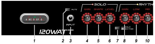
**1. ELECTRONIC TUNER:** The electronic tuner is active whenever the amplifier is turned on, providing constant, "real-time" tuning. The bottom row of LEDs indicate which note (string) is being tuned. The top row of LEDs provides directional queues to facilitate quick and precise tuning of your instrument. The indicated note (string) is properly tuned when only the center LED is illuminated.
