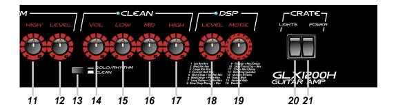
**19: DSP MODE:** Use this control to select one of the 16 built-in digital effects. A listing of the effects is shown on page 3 of this manual.
