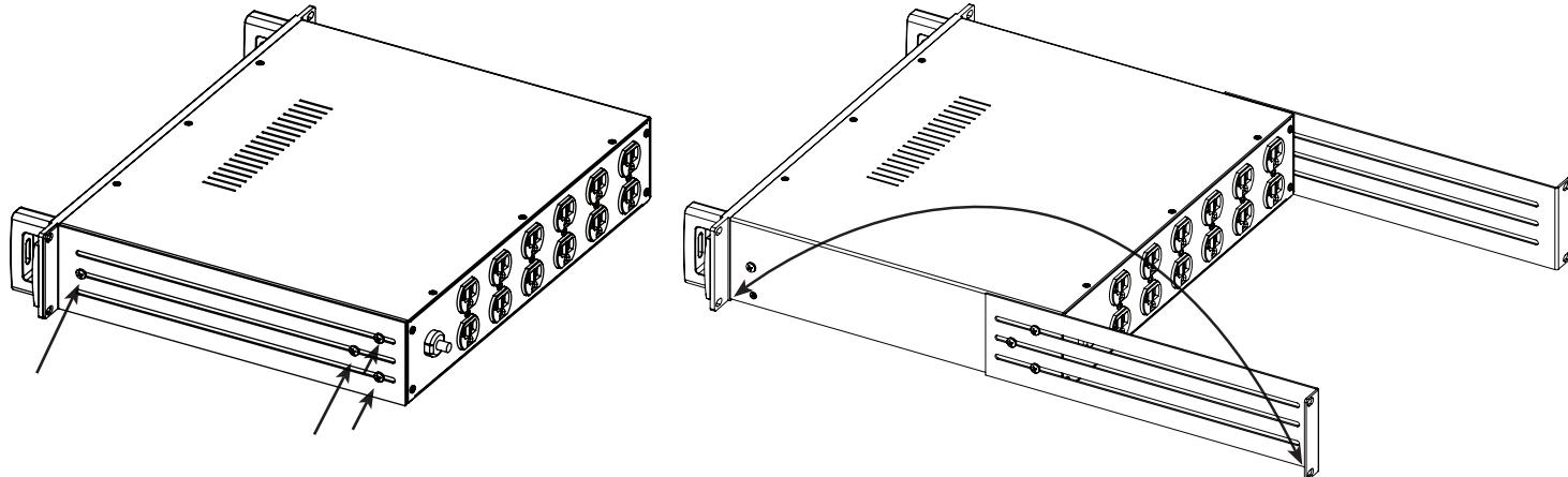
Remove the securing screws from the side and front portions of the P-2400 AR's adjustable rear rack ear and reinforcement side plate (located on either chassis side). Reverse the rack ears and re-attach to the P-2400 AR chassis (as shown on the right).
