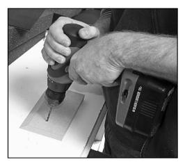
Use a screwdriver or cordless drill to fasten the wall cleat to the studs, or to appropriate anchors. Ensure the beveled side is up (see diagram).
