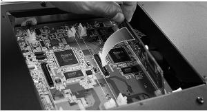
Never use excessive force when installing a circuit board. If it doesn't fit properly on the first attempt, remove the board and try again.
